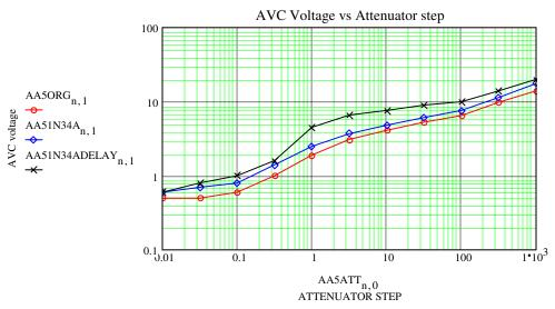
Output below 0.5V is dominated by grid leak bias voltage.
