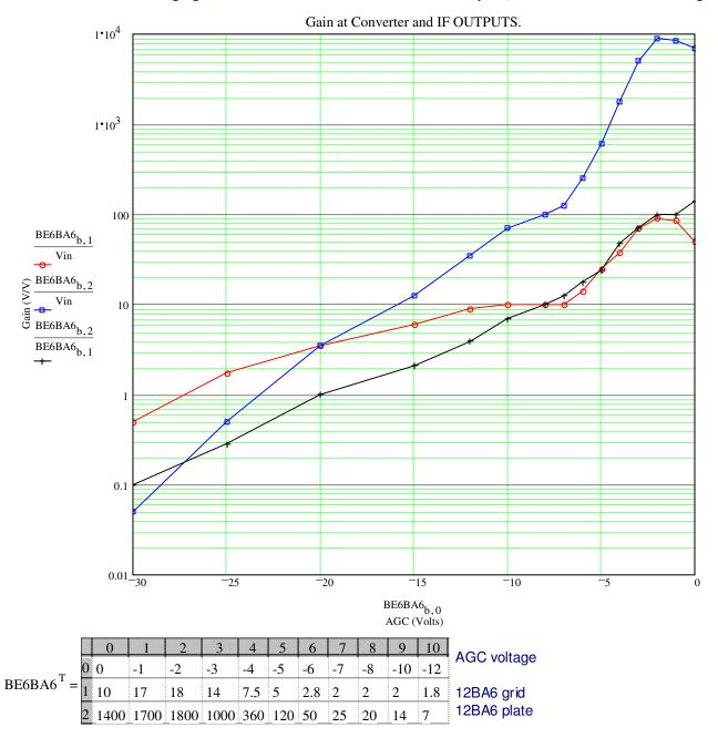
Voltage measurements conducted with 200mV p-p 1.2MHz at Ferrite terminals which was reduced for the higher gains to 20mVp-p or 2mVp-p.
