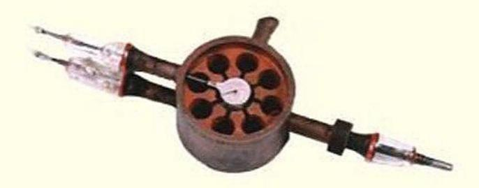
Pictured above is the 1189 C328 Cavity Magnetron. This is the second prototype ever to be produced. The Resonant Cavity Magnetron, produced from 1940, originated from a design devised by two Birmingham scientists, Randall and Boot. GEC played a leading part in its development and production through its work at the Hirst Research Laboratories, Wembley, London. The cavity magnetron's application to radar was a major factor in the Allied victory in World War II.
