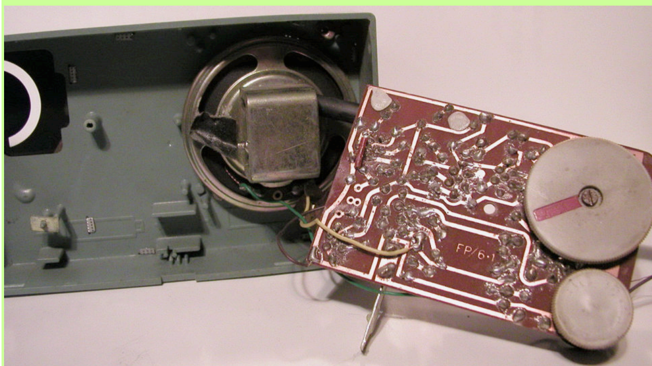
Fig. 14 - Chassis of KANYO, view from the printed circuit side
