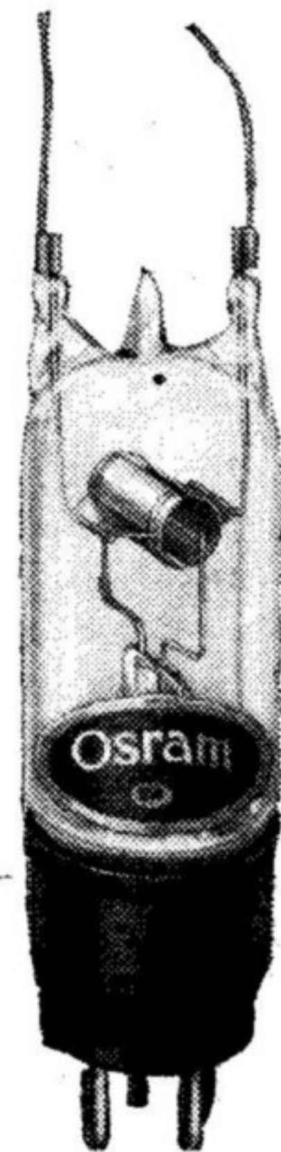
Fig. 7.—Construction of a split anode Magnetron, as used at extremely high frequencies.
