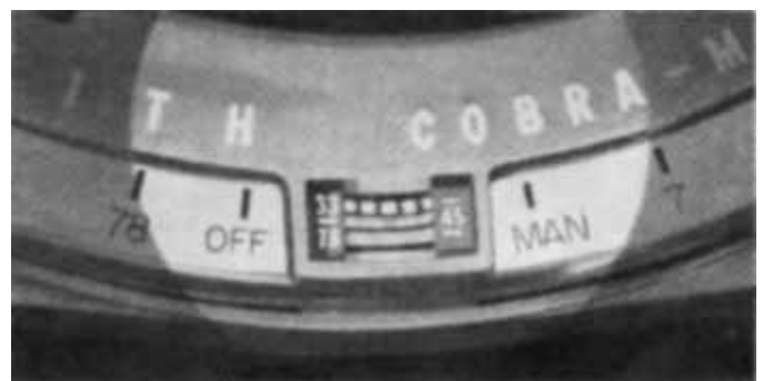
Among Zenith high fidelity advances are the speed control continuously variable from 10 to 85 rpm and the strobe-scope indicator . Without them true high fidelity is impossible.
