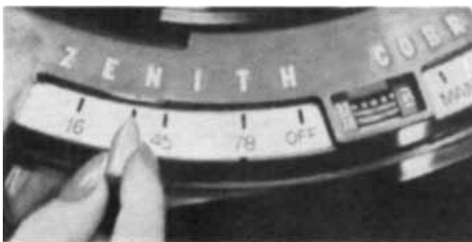
Among Zenith high fidelity advances are the speed control continuously variable from 10 to 85 rpm and the strobe-scope indicator . Without them true high fidelity is impossible.
