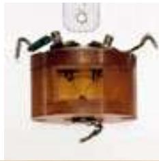
First European transistor constructed in June, 1948 at the Semiconductor Laboratory of P & S Westinghouse in Paris, France by H. F. Mataré
