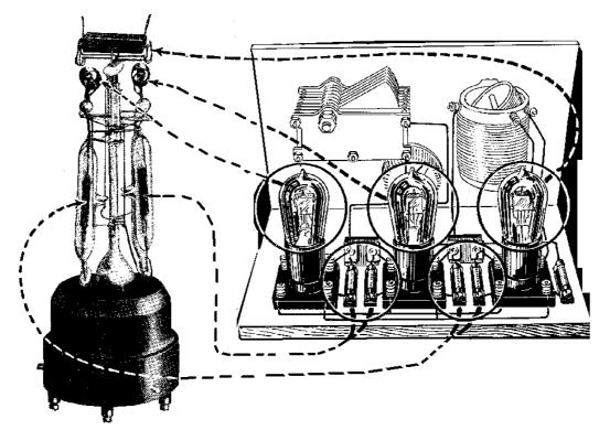
This diagram indicates the number of tubes and their connecting apparatus that Dr. Loewe has condensed into one of his new vacuum tubes.
