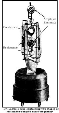
amplification It may bee seen upon inspection of the illustrations of the tubes, that the one which contains the three tube elements is of construction quite different from the
