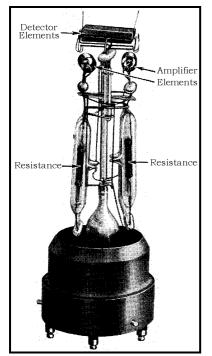
In this tube there are a detector and two stages of A.F. amplification
