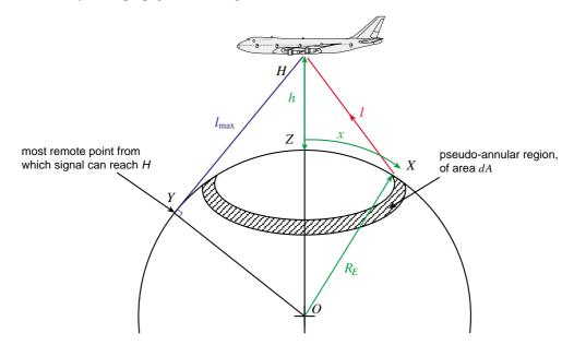
The aircraft is flying at height h above the Earth, and is at point H vertically above Z. Signals from point X travel to the aircraft along the slant path XH, whose length l is given by:
