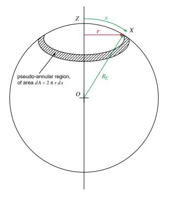
The Figure above shows an annulus-like infinitesimal ring of area dA on the curved surface of the Earth, whose radius is  $R_E$  and whose centre is at O. The ring is at distance x from the receiving point Z (as measured round the curved surface), and has a radius, measured from OZ, of r. The angle  $\angle ZOX$ , i.e. half that subtended at O by the ring, is  $\frac{x}{R_E}$  radians and so r is given by:
