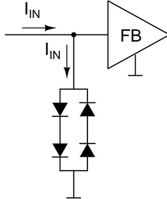
Figure 4: Diode clipper as voltage limiter
