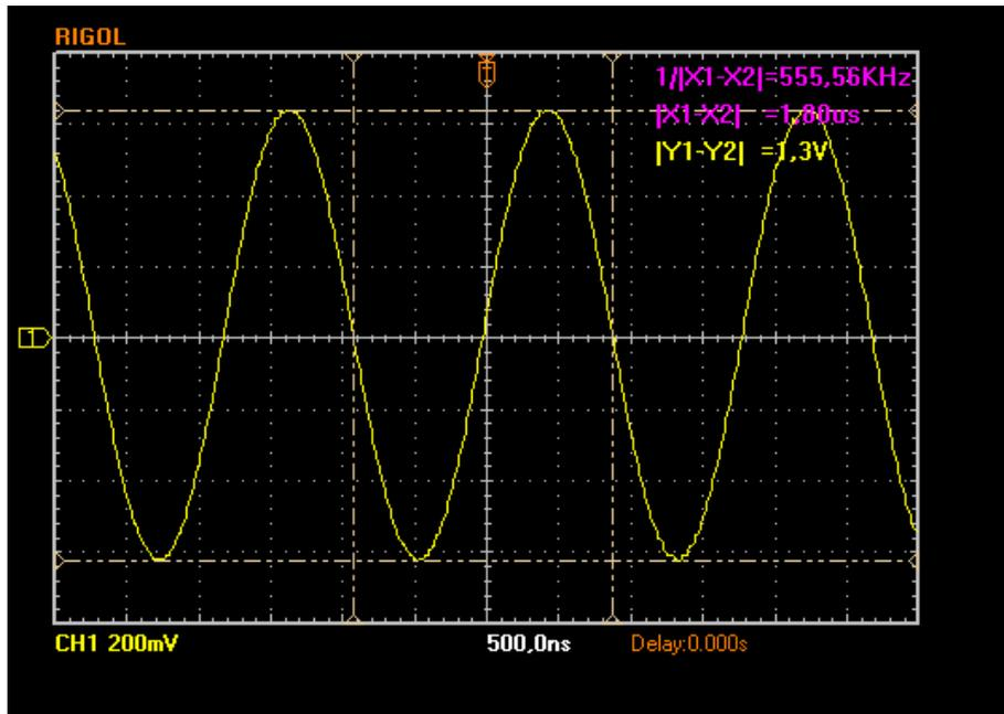
Figure 8: Nearly harmonic oscillations for  $R_E = 10\text{k}\Omega$
