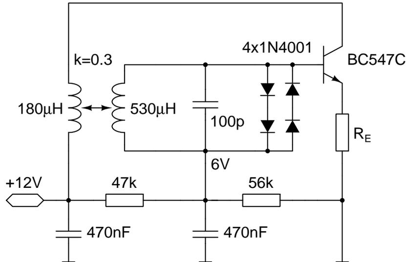
Figure 7: Practical LC-oscillator with amplitude limiting
