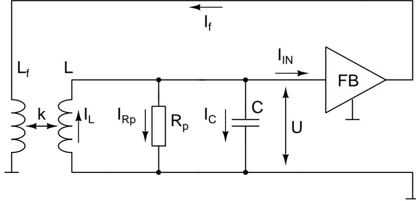
Figure 2: Tuned input, inductive feedback oscillator
