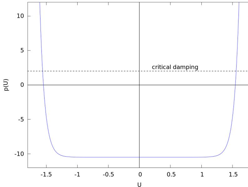
Figure 5: Damping due to diode clipping
