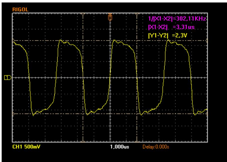
Figure 9: Relaxation oscillations for  $R_E = 560\Omega$
