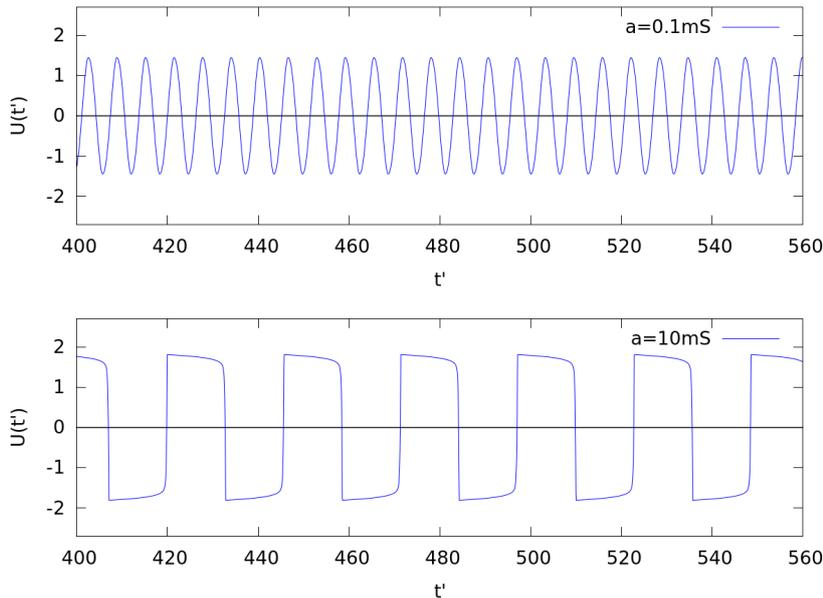
Figure 6: LC-oscillator harmonic and relaxation oscillations
