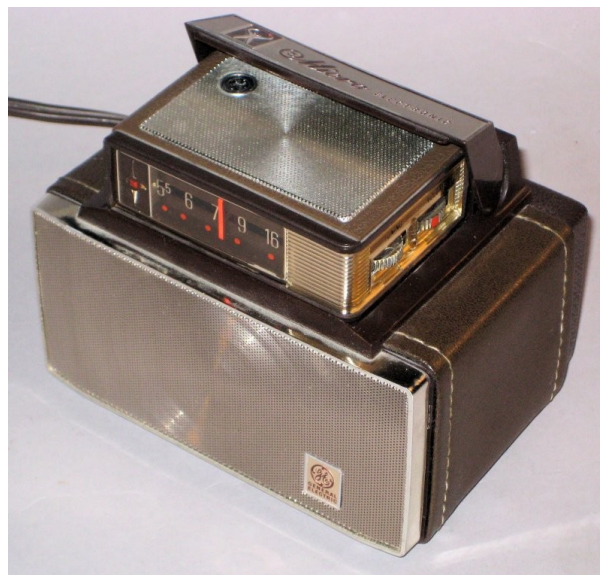
Fig. 2: General Electric P 1740 . General Electric P 1740. First IC (pocket) receiver of the world in 1966. The receiver (above) is removable and works then as usual pocket radios; in the lower part a large auxiliary loudspeaker and the accumulator charging unit are accommodated. There was also a version with alarm clock.
