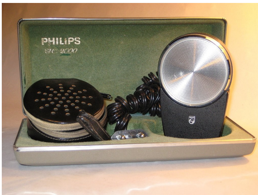
Fig. 5: Philips IC 2000, the first European IC-receiver from 1967 with recharging unit, leather carrying bag and case. Dimensions: radio 7,2 x 7,5 x 3 cm, case 21,8x10,5x4,3 cm.
