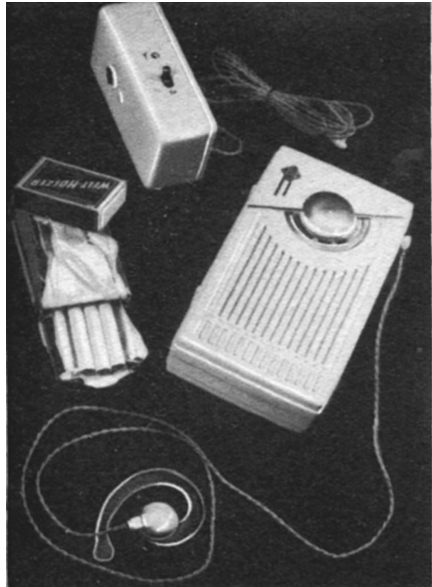
Illustration 3: Transistor pocket receiver Telefunken TR 1; on the left top, the power supply unit
