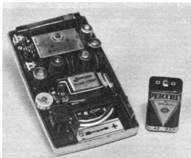
Illustration 2: Inside view of the 6 transistors Telefunken pocket receiver TR 1, beside the 22,5V battery
