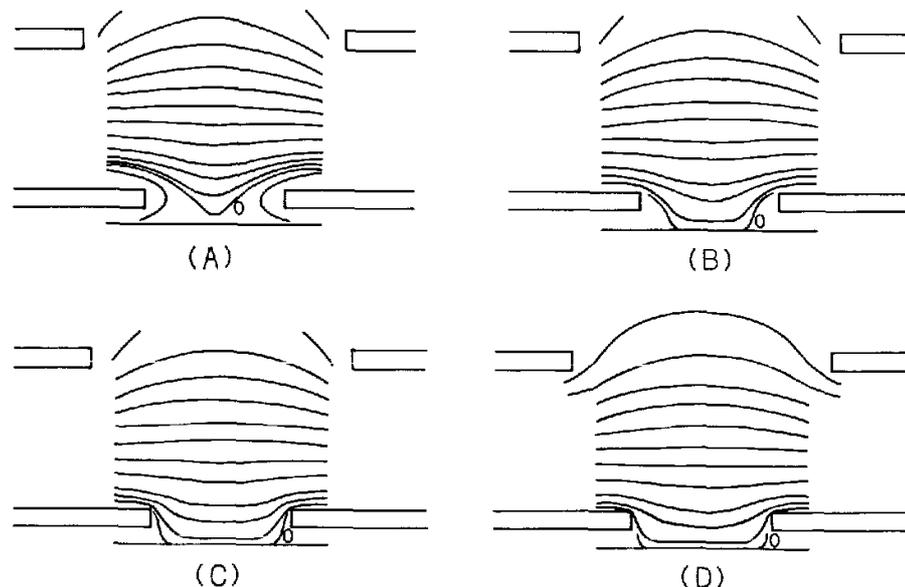
Fig. 3-4. Equipotential line plot for various grid bias.
