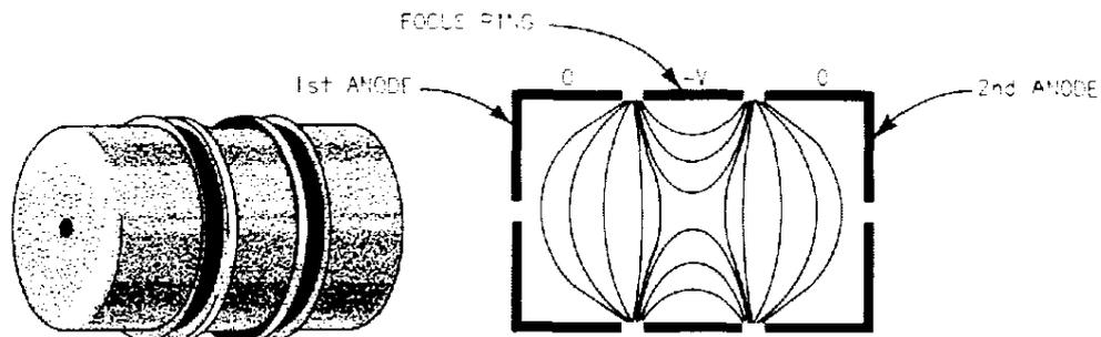
Fig. 5-1. Equipotential line plot within focus lens.
