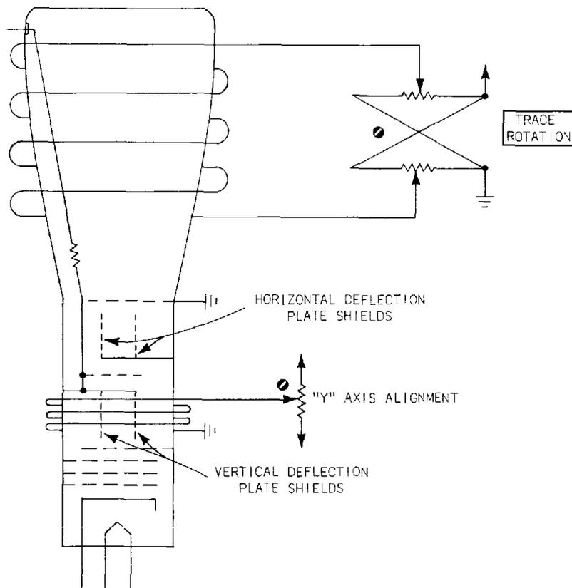
Fig. 18-3. Y-axis alignment control.
