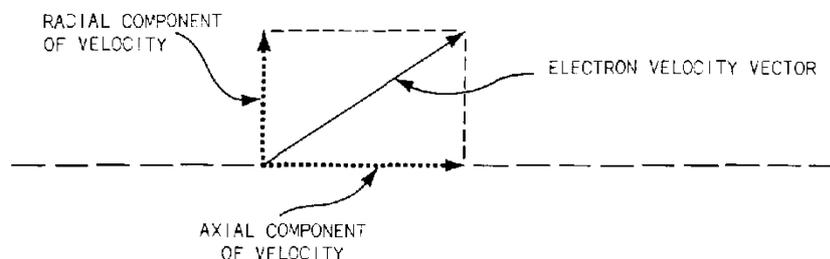
Fig. 2-1. Velocity components.
