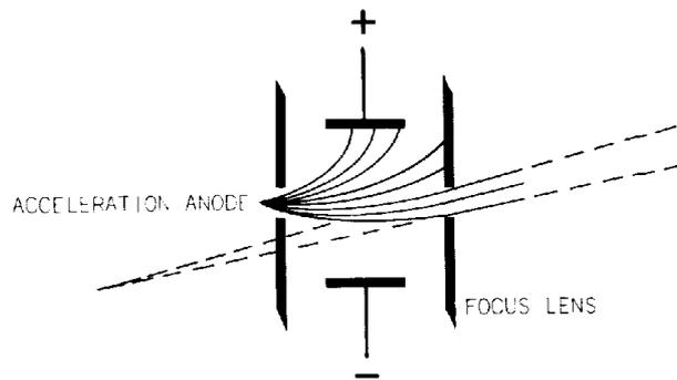
Fig. 4-4. Single deflection unblanking plate.
