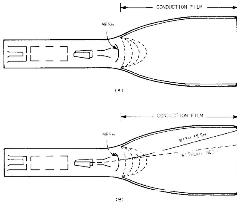
Fig. 7-5. Mesh-type PDA CRT.
