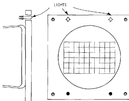
Fig. 17-2. External graticule and its illumination.
