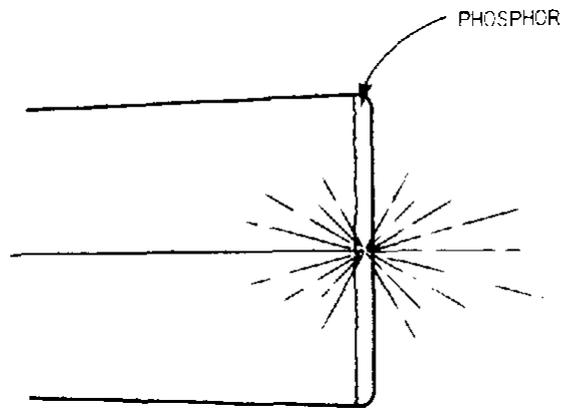
Fig. 15-1. Light scatter of non-aluminized CRT.
