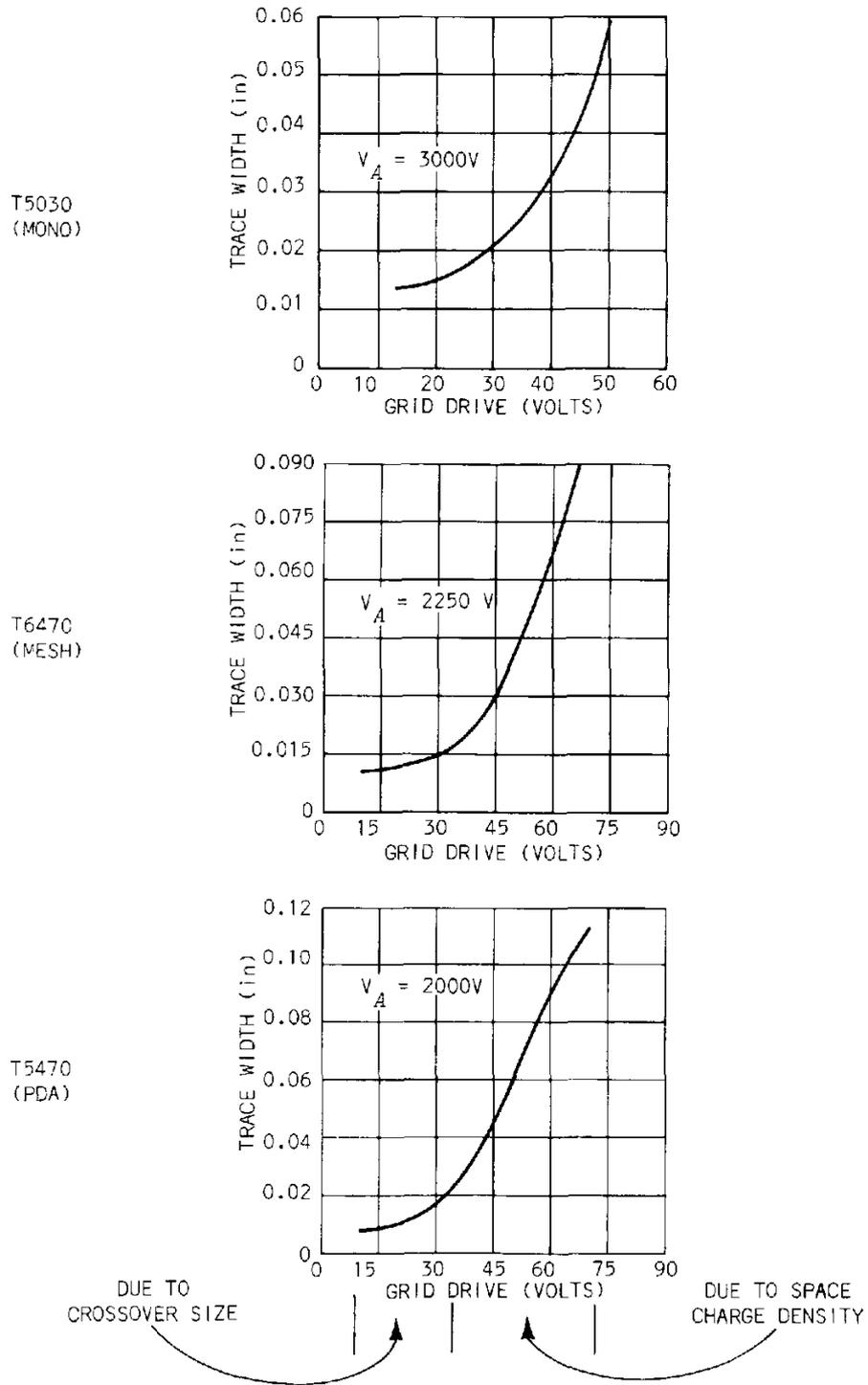
Fig. 8-3. Grid drive vs trace width.
