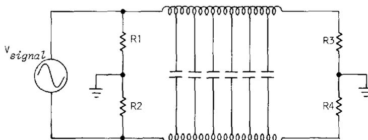
Fig. 6-8. Push-pull distributed deflection schematic.
