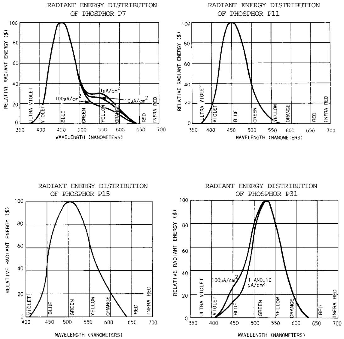
Fig. 12-1. Radiant energy distribution of P7, P11, P15, P31 phosphors.
