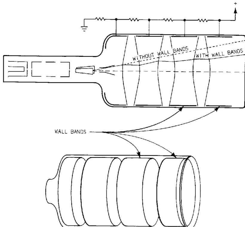
Fig. 7-1. Aquadag applied as wall bands.
