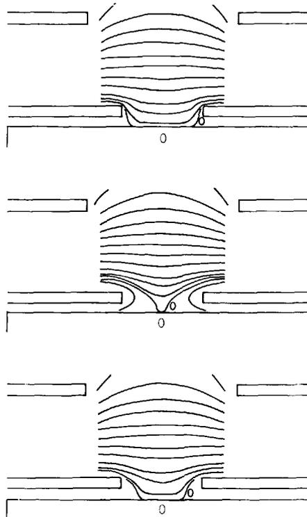
Fig. 3-7. Equipotential line plot for various grid bias.
