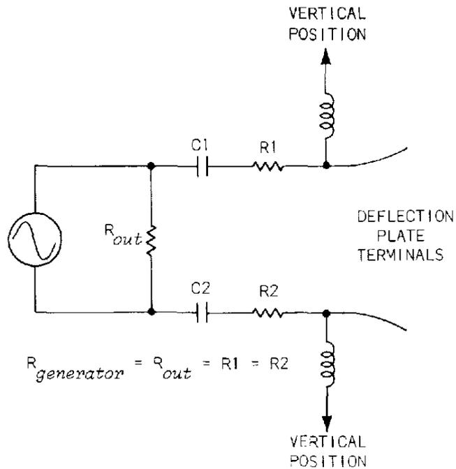
Fig. 6-28. Direct connection network.
