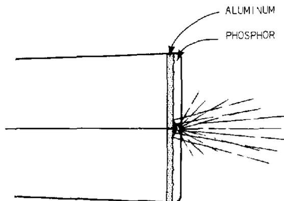
Fig. 15-2. Reduced light scatter of aluminized CRT.
