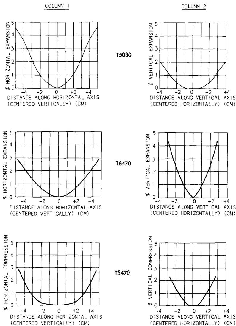
Fig. 6-14. Deflection-linearity characteristics.
