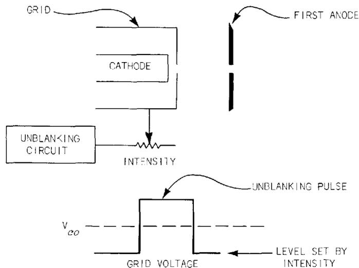
Fig. 4-1. Grid unblanking.
