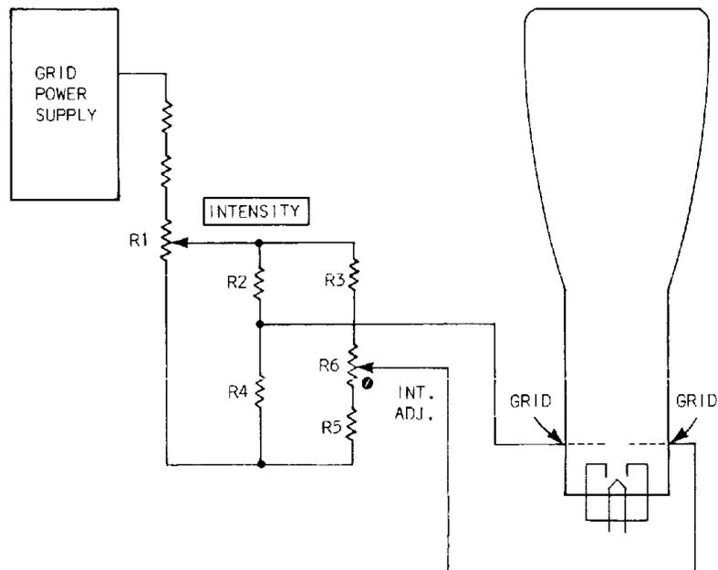
Fig. 20-3. Intensity Balance control.
