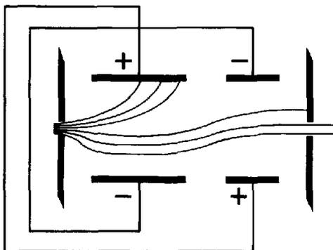
Fig. 4-6. Correction for single plate deflection unblanking problems.
