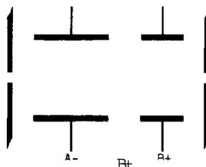
Fig. 4-3. Typical deflection unblanking plates.
