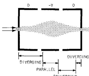
Fig. 5-2. Electron trajectory within focus lens.
