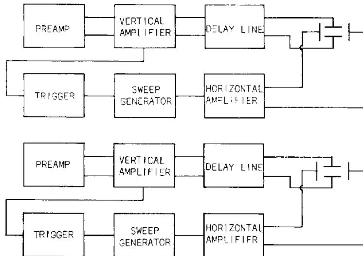
Fig. 20-1. Block diagram of dual-gun oscilloscope.
