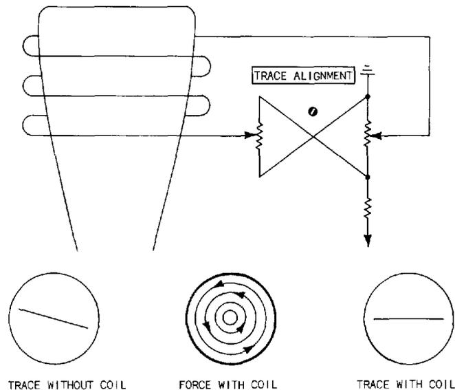
Fig. 18-2. Trace alignment control.
