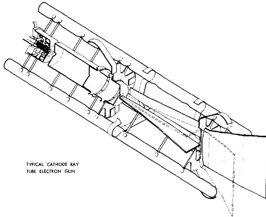
Fig. 1-2. CRT electron gun.
