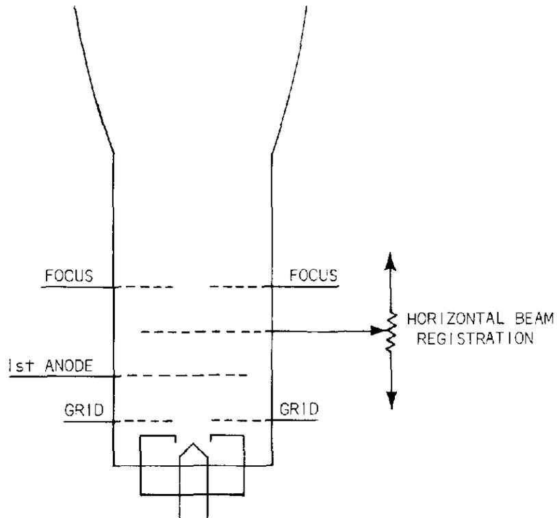
Fig. 20-5. Horizontal beam registration control.
