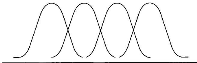
Fig. 8-6. Trace width measurement using 50% brightness points.
