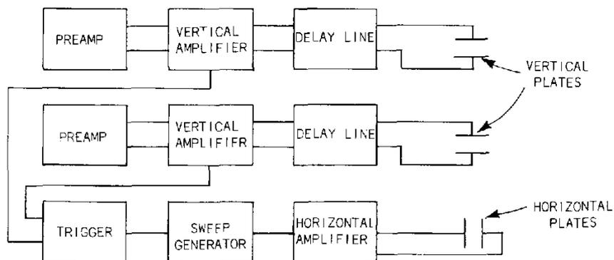
Fig. 19-1. Dual-beam oscilloscope block diagram.
