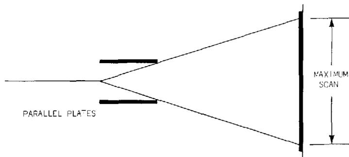
Fig. 6-3. Maximum scan using parallel plates.
