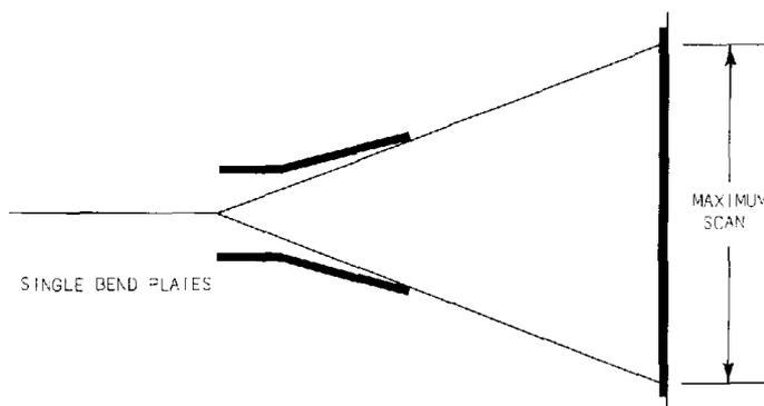
Fig. 6-4. Maximum scan using bent plates.
