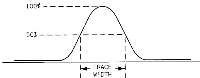
Fig. 84. Gaussian distribution of trace width.
