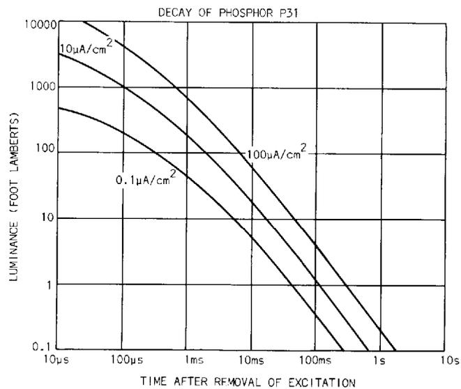
BUILD UP: Approximately 500 microseconds to 90% at  $10\mu\text{A}/\text{cm}^2$ .
