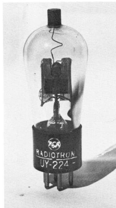
Early production model UY-224. Note fork-shaped screen assembly.
