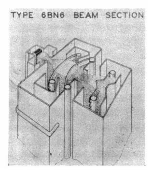
Fig. 2—Type 6BN6 beam section
