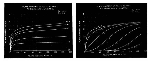
Fig. 12—Plate current vs. plate voltage No.1 grid parameter Fig. 13—Plate current vs. plate voltage No. 2 grid parameter
