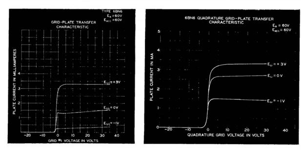
Fig. 3—Grid-Plate Transfer charateristic
