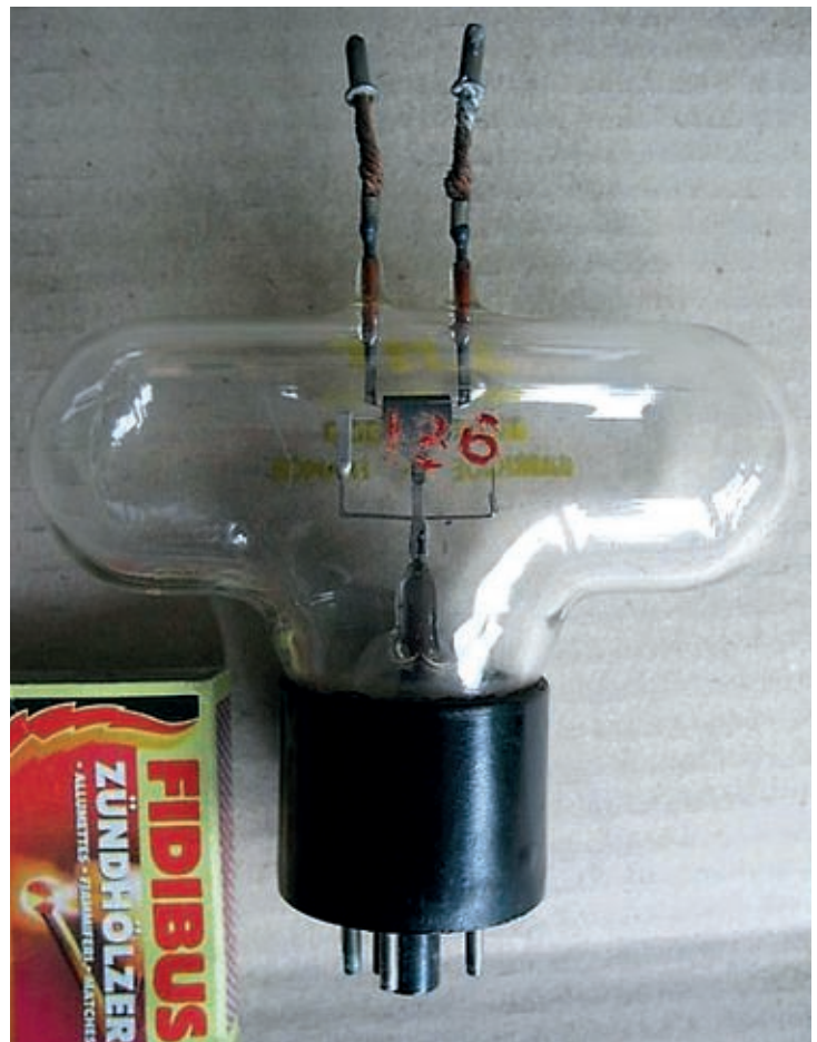
Fig. 5 Spiral grid tube type 3036 made by LMT.
