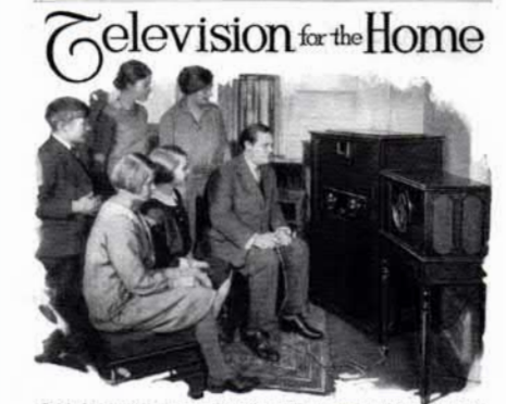
Behind a Little Three-Inch-Square Aperture, the Moving Picture from the Radio Studio Appears. While the Viewer, with a Post Office in His Hand, Keeps the Picture Inconspicuous... GROUPS of people sitting in various homes at Schenectady, N. Y., a few weeks ago, saw the performers in a distant broadcasting studio fit across a tiny screen, and from the loud speaker of a radio set heard them talk. Television, a laboratory plaything that has interested scientists for several years, had arrived. A large, square cabinet, built somewhat like the bigger talking-machine models, is the first home receiver for radio-transmitted images. The dial of a receiver protrudes from its middle, and above them, at the eye level of the seated spectator, appears a three-inch-square window, behind which is the screen on which the images are formed. The one great problem that has perplexed television experimenters for years—how to synchronize the transmitter and the receiver—was solved by simply ignoring it. Instead of all the elaborate, and very expensive, equipment necessary to keep the whirling disk of pictures that paints the image on the receiver screen in absolute step with the corresponding mechanism that transmits the original
